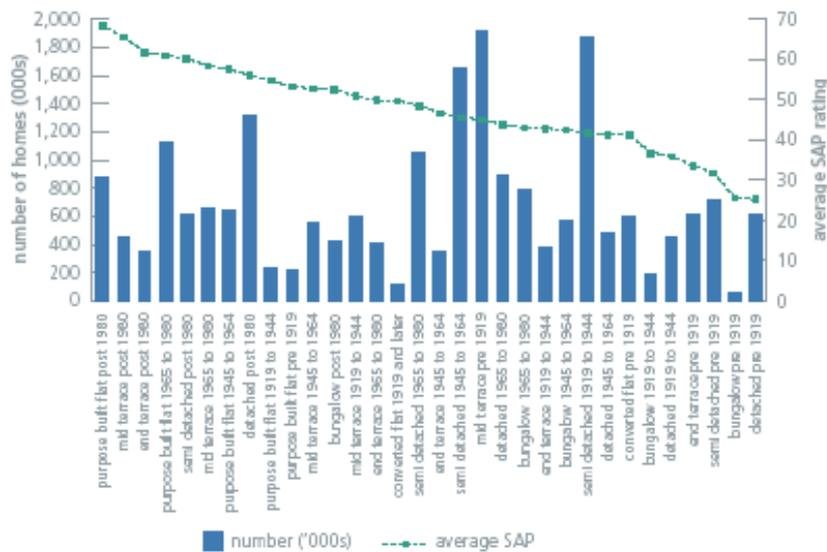
Figure 1. Average SAP and size of stock by housing types and age combined
